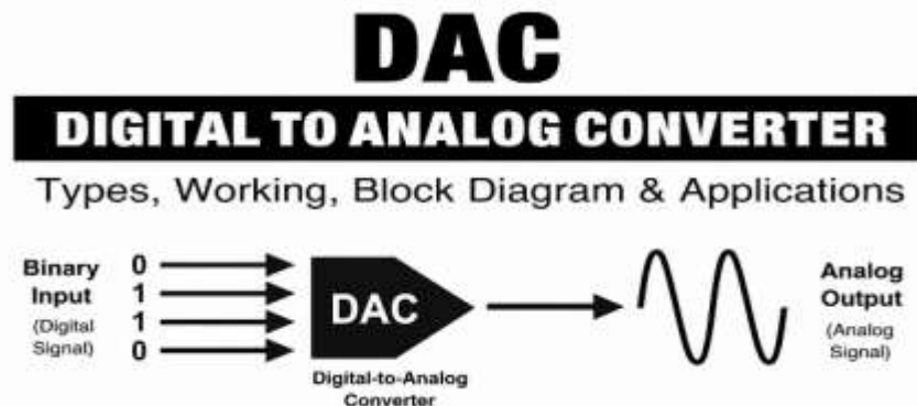
Figure 1. Basic digital-to-analog conversion from a binary input to an analog output waveform.
